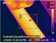
Infrared thermography is a thermal imaging technology that analyzes equipment heat signatures and can identify typical electrical problems, mechanical malfunctions, and potential belt failures. (*Image courtesy of Blue-Cardinal.*)
